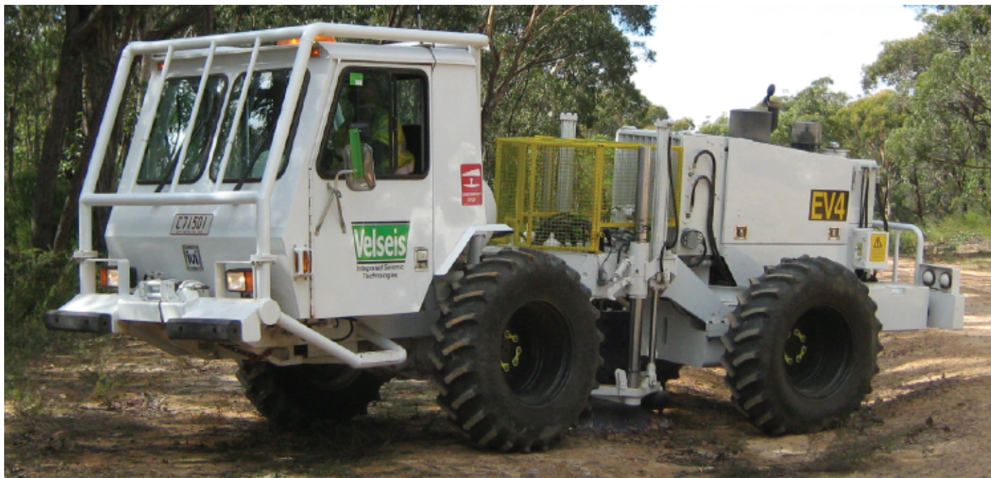
FIGURE 1: 3D seismic survey truck-mounted vibroseis unit called the EnviroVibe minibuggy.
