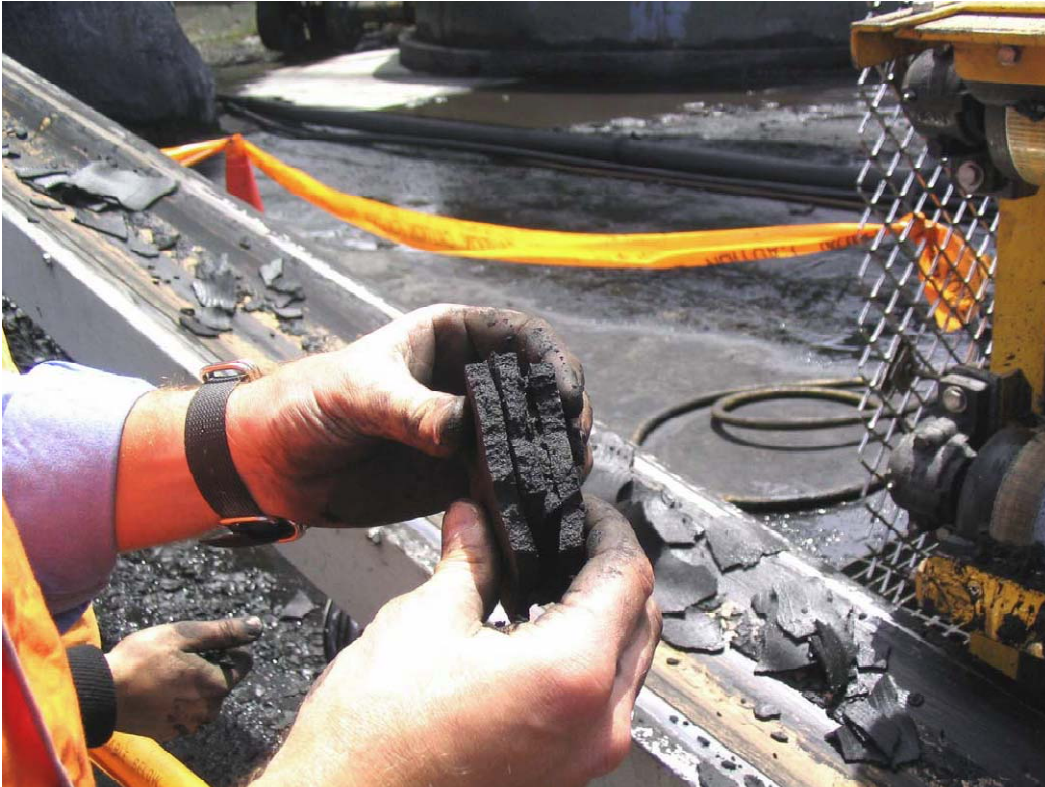
Figure F-6 Final belt press filter cake prior to disposal
